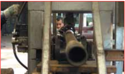
A straightening process then insures the rods are true and accurate.
