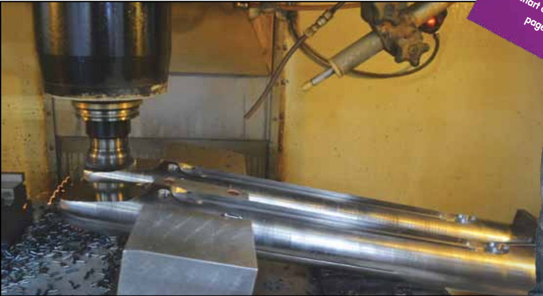
CNC machine milling face on housing before milling threads for bolt-on blade feature. Threads are milled to the bottom of the hole allowing more thread engagement for the bolts and stronger connection.
