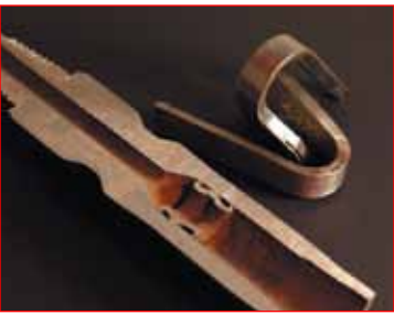
A cross section of the inertia weld shows the strength of the weld.
