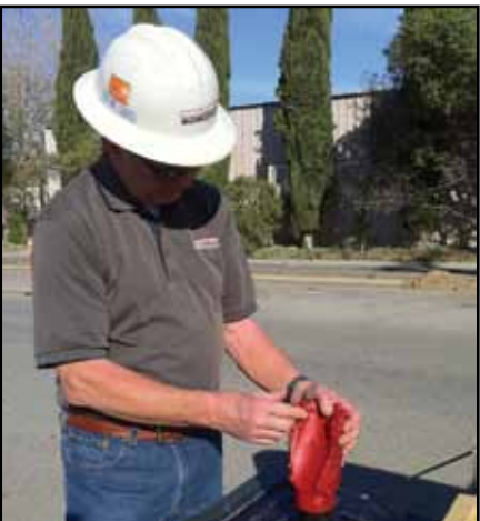
Above: Melfred Borzall engineer examines the Iron Fist on the job site. Below: Minimal wear on the Iron Fist after a 300 ft. bore in rocky soil conditions.
