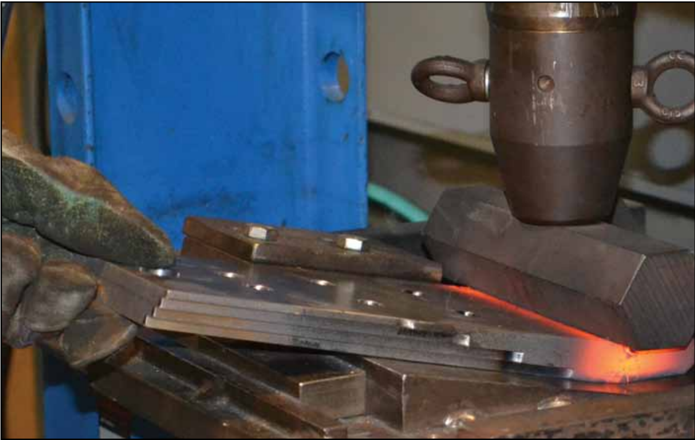
Below: Heated blade in the process of being bent before going to heat treating.
