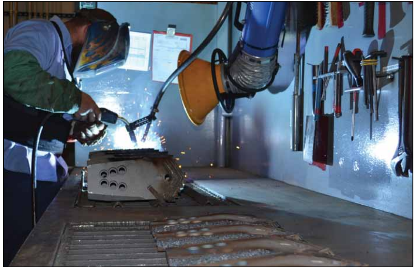
Applying hardfacing to the Ultra Bit 3 blades.
