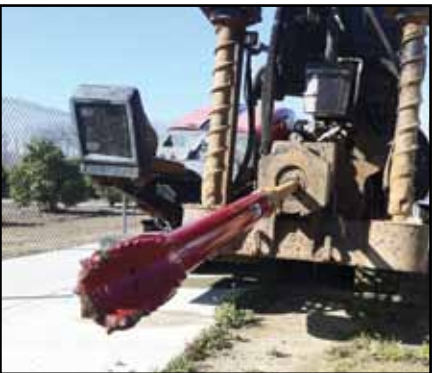
Above: Melfred Borzall engineer examines the Iron Fist on the job site. Below: Minimal wear on the Iron Fist after a 300 ft. bore in rocky soil conditions.
