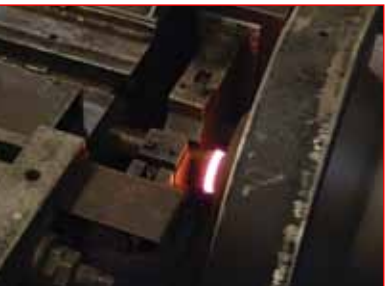
Using inertia welding, the threaded connection is "fused" to the forged tube to make a superior connection.
