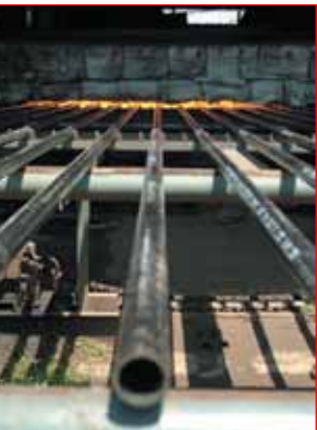
The rods are strengthened through a careful heat-treating process.
